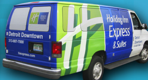
Here is a Partial Wrap example where the entire front-section of the vehicle was left unwrapped. Simple die-cut lettering was applied to the doors for location-specific information. Window Perf vinyl was added to all windows so people could see out of this Shuttle Van.
