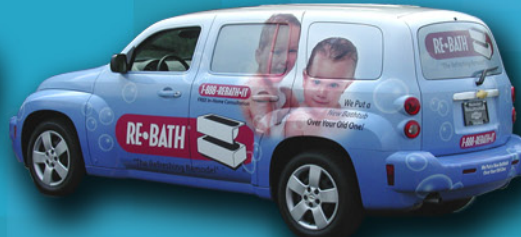
This is a perfect example of a Full Wrap. Notice how all areas of the vehicle received graphics including the Windows (using Window Perf material) and the roof.
