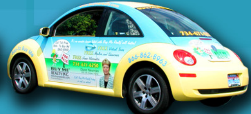
This VW started off bright yellow. We added a Partial Wrap between the doors and die-cut vinyl lettering around the wheel wells for the phone number.
